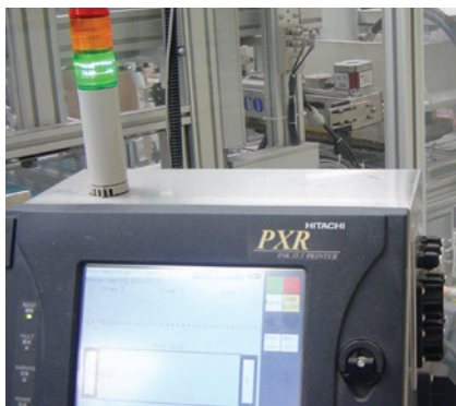
All newly installed ink-jet coders are equipped with a 10.4-in. color, backlight LCD HMI designed for ease of operation.
