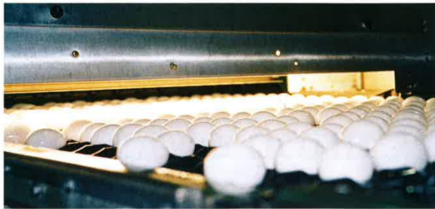
Eggs move through a blood-detection system, above, that shines a light through the eggs to see if there are any blood spots within. Egg cartons are coded by a four-line ink-jet printer, at top of page, with the Julian date, plant number and sell-by date.
