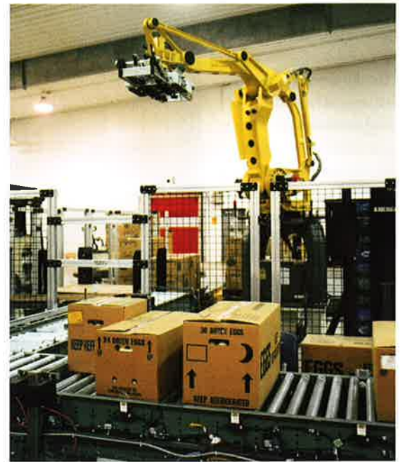
A portion of the cases are palletized through the use of a four-axis, electric, servo-driven robot that can handle four different case sizes at one time.
